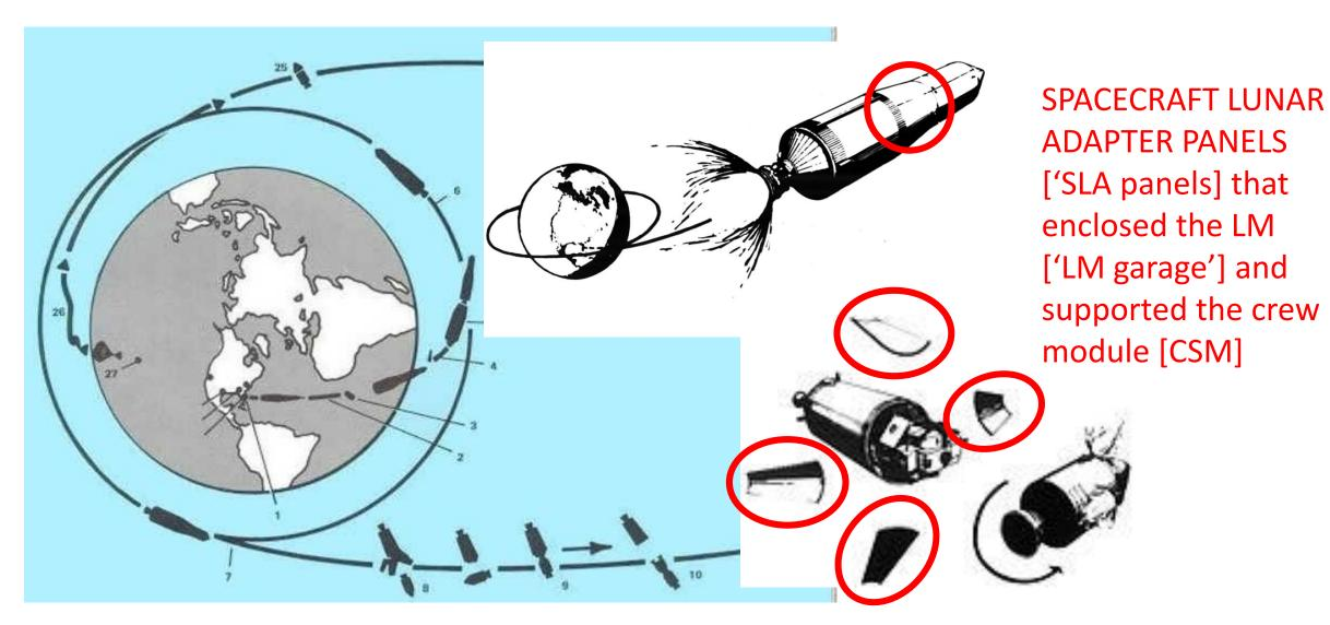
Detail – S4B thrusting, then separation, 'transposition', docking to LM, extraction from launch shroud
