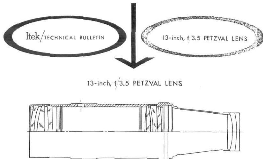
Itek's 13-inch, f/3.5 Petzval lens is an extremely high acuity lens that provides a high contrast AWAR of over 235 lines per millimeter. Low contrast AWAR is over 150 lines per millimeter. Performance is excellent in either white light or over more limited spectral regions.
