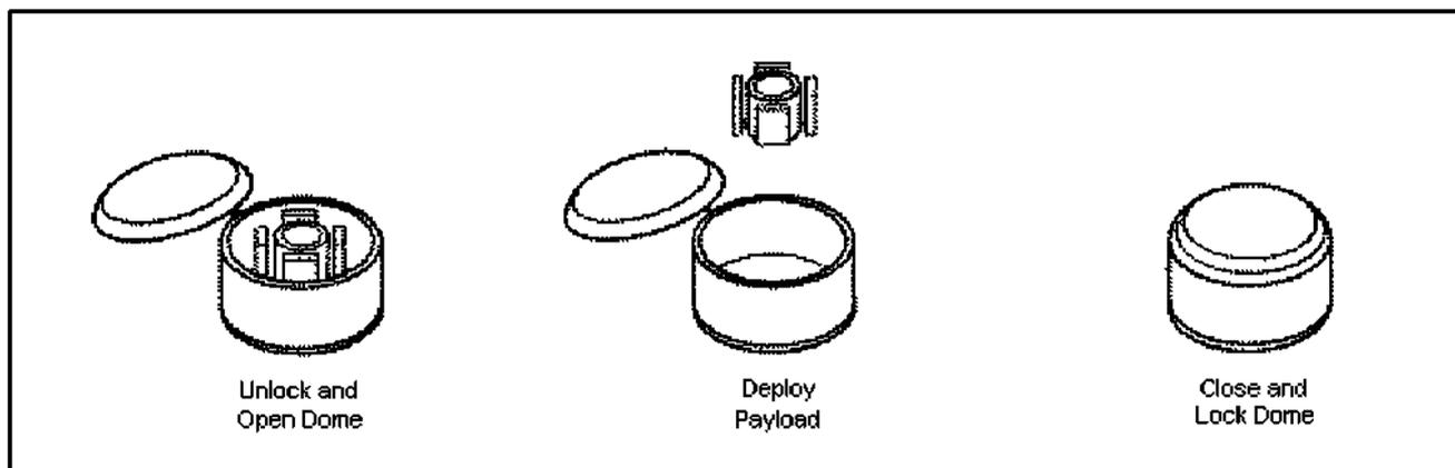
**Figure 4-2. Axial Payload Deployment – Standard Payload Module (SPM)**
