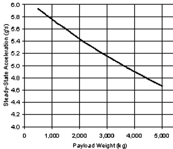
**Figure 6-1. Maximum Axial Acceleration**
