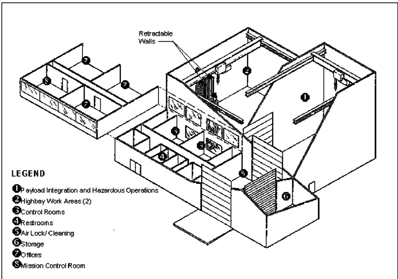
**Figure 8-4. Payload Processing Facility (PPF)**
