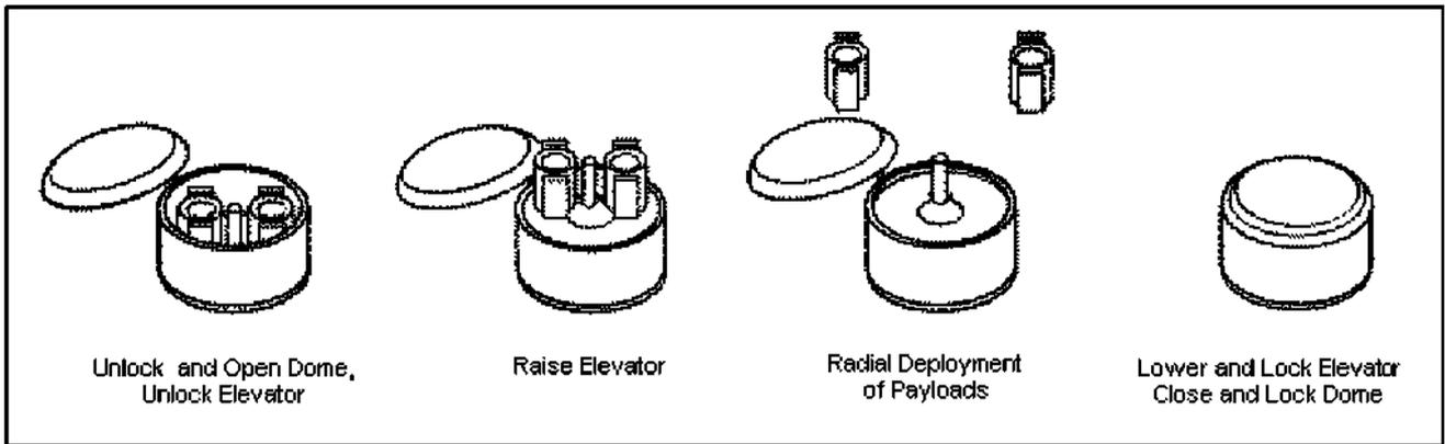
Figure 4-4. Axial Payload Deployment – Extended Payload Module (EPM)
