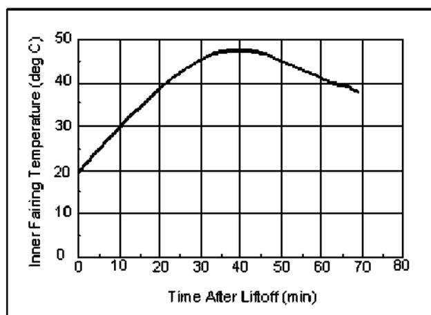
Figure 6-5. PM Inner Surface Temperature
