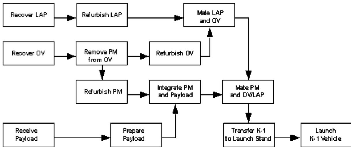
**Figure 8-8. Launch Process Flow**
