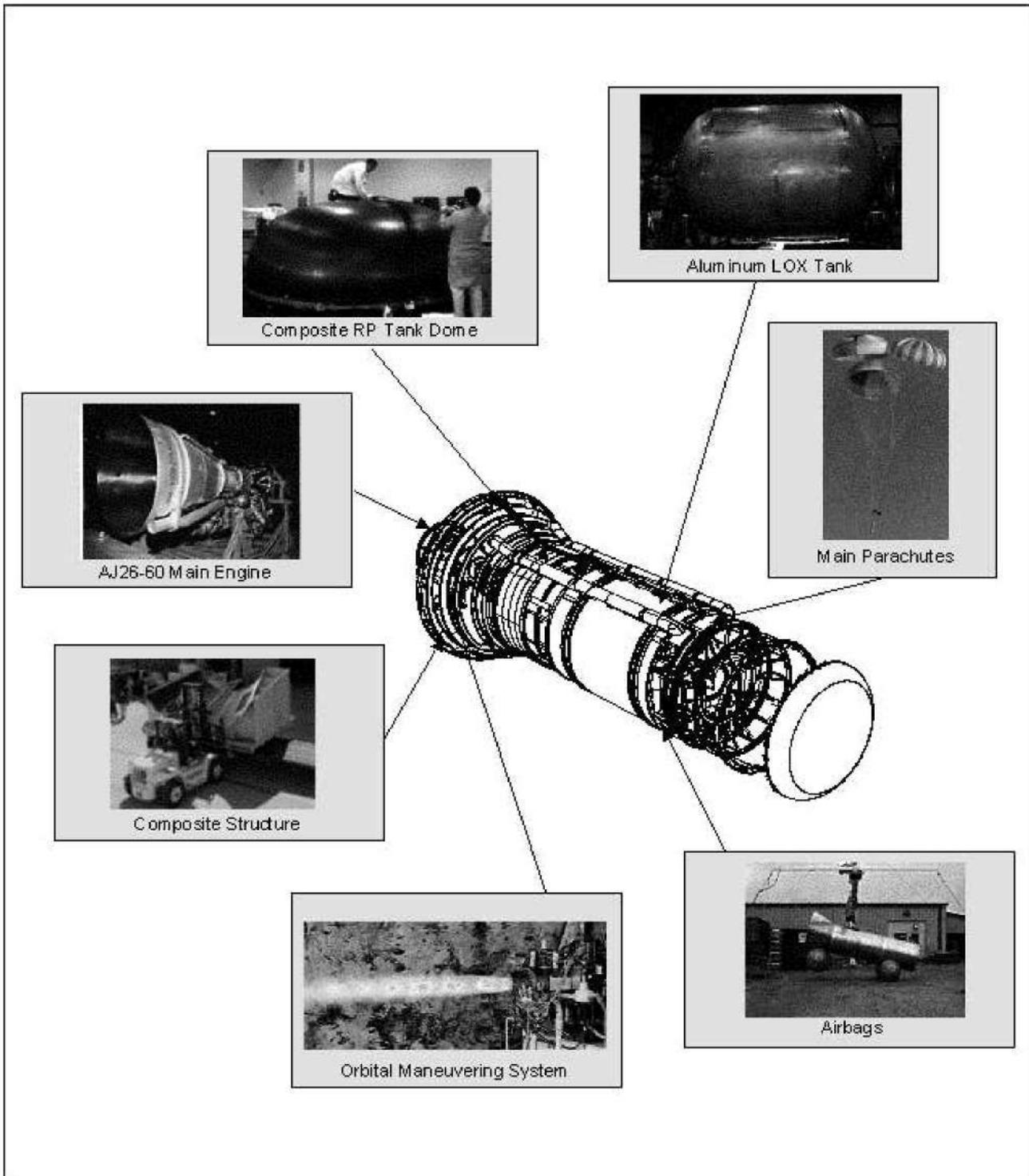
Figure 2-3. Orbital Vehicle (OV) Overview
