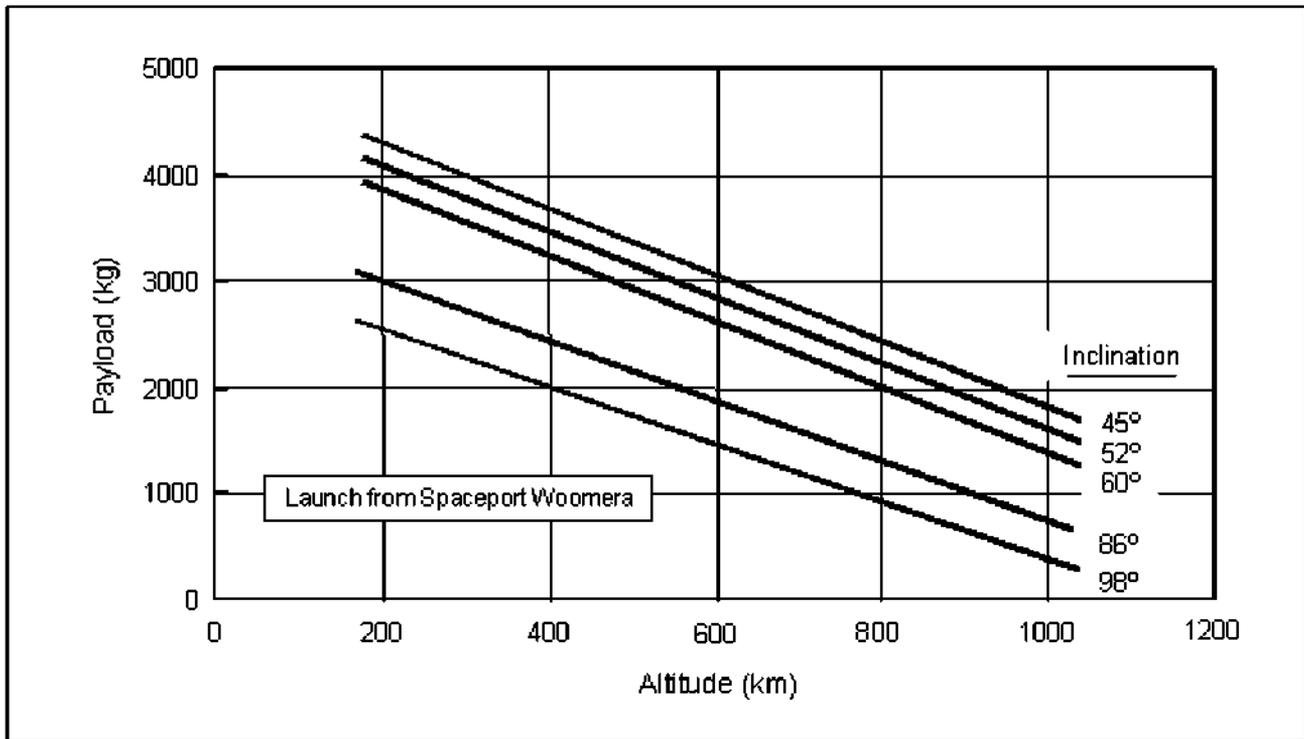
Figure 3-7. Circular Orbit Performance with EPM
