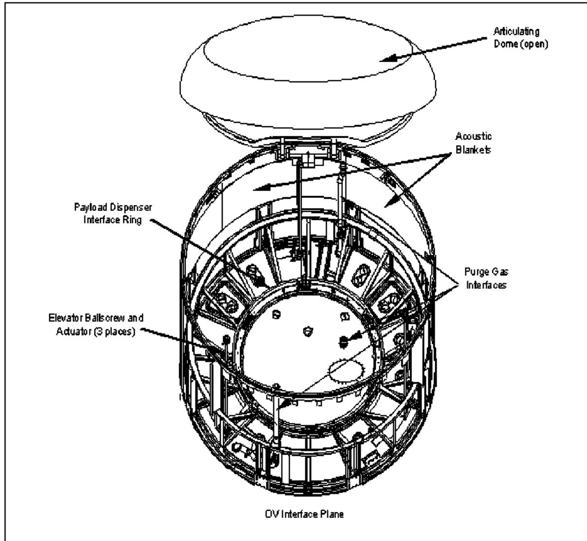
**Figure 4-1. Standard Payload Module**
