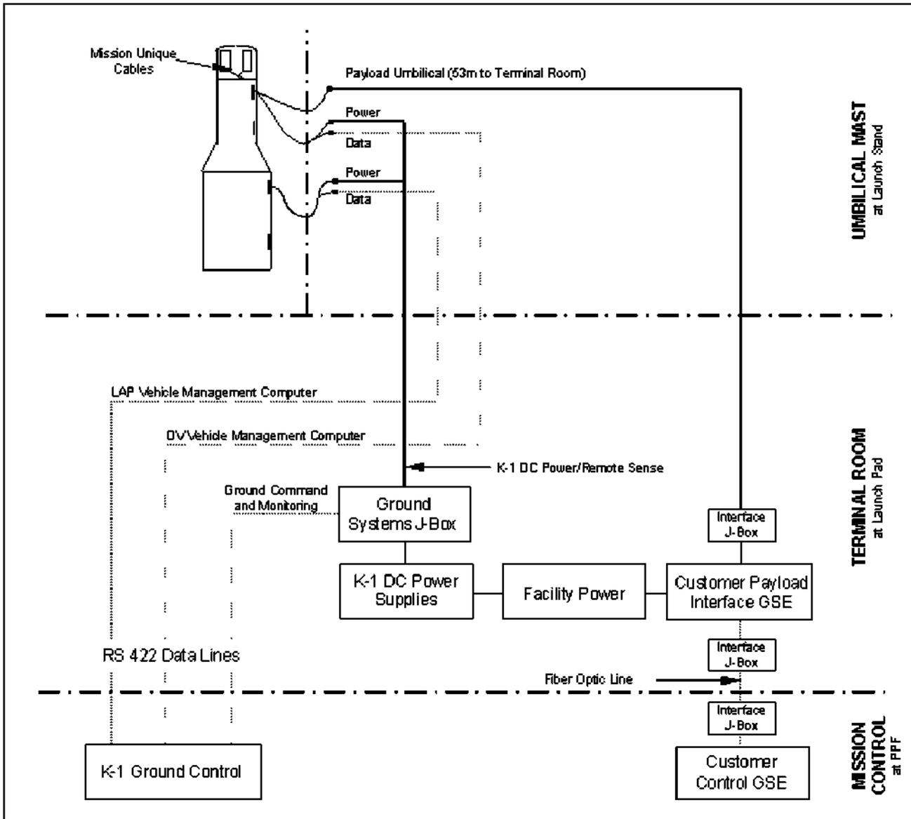
Figure 5-2. Customer and Launch Control Electrical Interfaces
