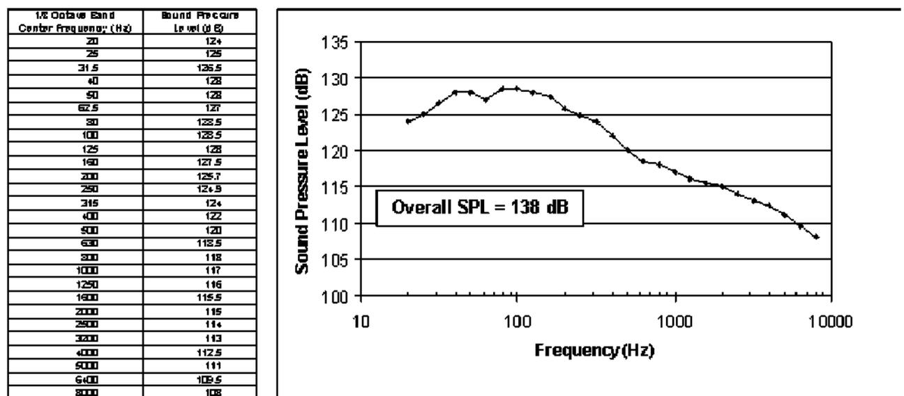
Figure 6-2. Acoustic Environment (1/3 Octave Band Level)
