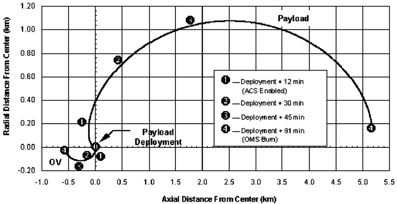
Figure 3-5. Post-Deployment Clearance
