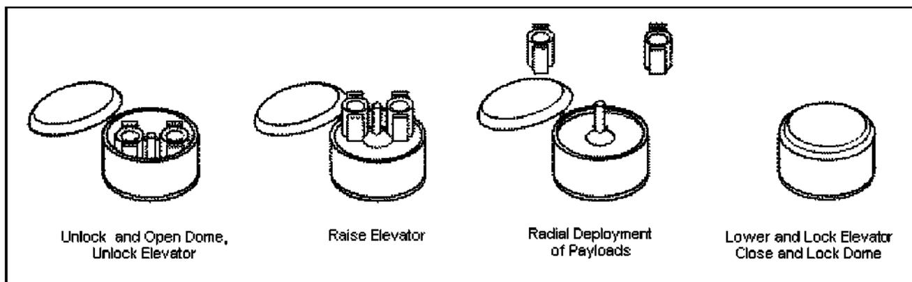
**Figure 4-3. Radial Payload Deployment – Standard Payload Module (SPM)**
