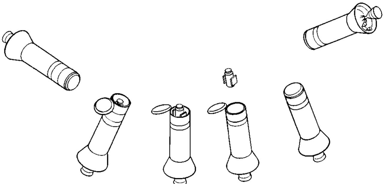
Figure 3-4. Payload Deployment Sequence
